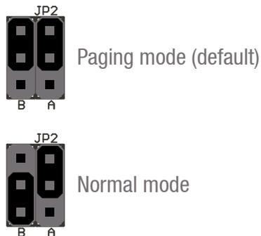
**Paging mode:** At power-on, all relays will be activated and will be switched to background music mode. In case of power interruption (emergency situation) the relays will return back to their idle state. This configuration is recommended when using the ARU20x in music / paging announcement systems.
