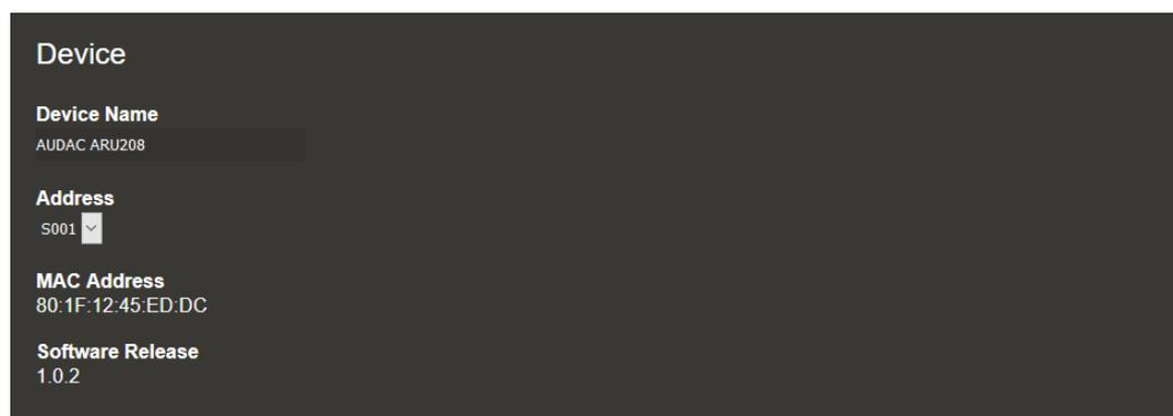
The device address is an unique address which shall be used when multiple units are daisy-chained with each other and addressed through a single IP address. Each device in the chain should have an unique device address which is selectable between 'S001' and 'S099'.
