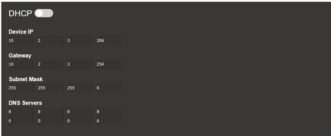
The DHCP function is standard switched off and can be turned one by clicking and enabling the corresponding indicator.
