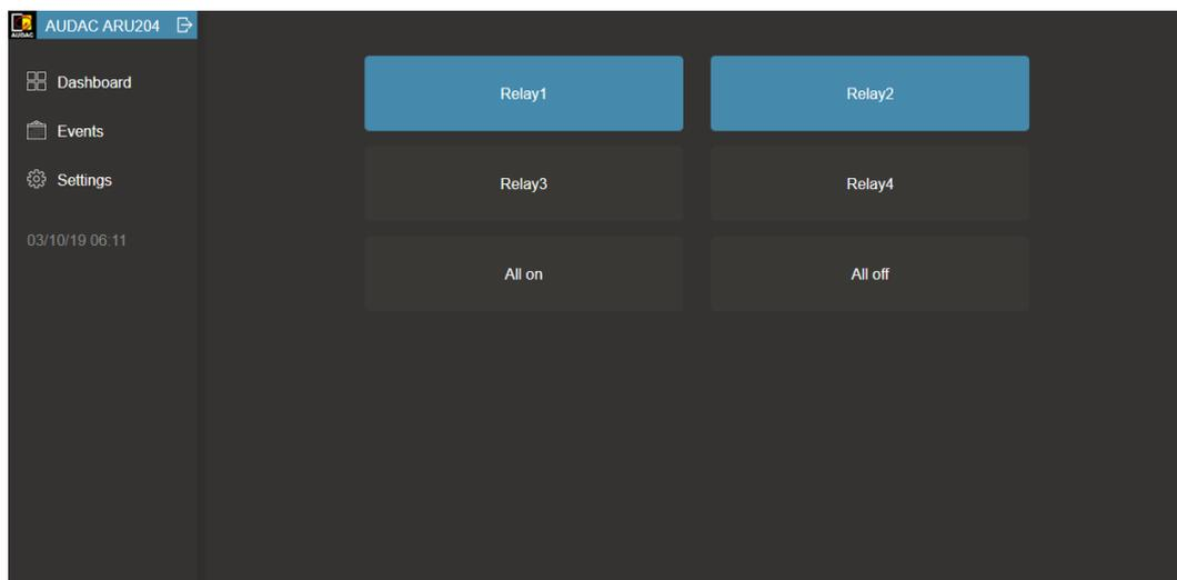
The text inside the relay knob is default shown as 'Relayx' where x represents the number of the corresponding relay (1 up to 4 for ARU204 or 1 up to 8 for ARU208). This text can be adjusted according to customers preferences, allowing to create a more clear and intuitive interface for the user.
