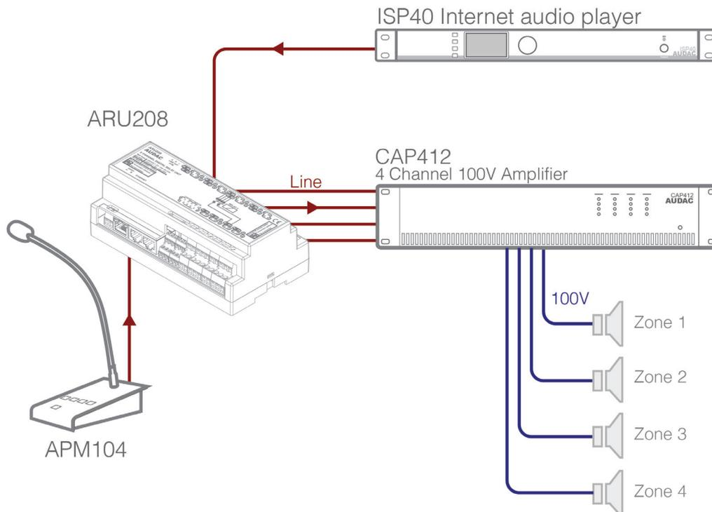
The above diagram shows an example of a simple and basic setup with an APM1xx paging console in an analogue paging setup, combined with an ARU20x relay unit. Besides the APM1xx paging console, a background music source (ISP40 in this typical setup) is connected.
