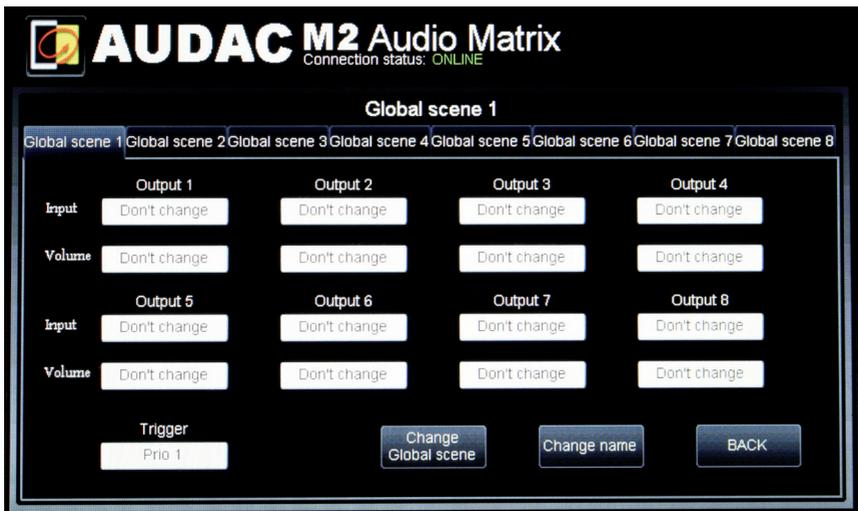
A global scene are preset settings which are enforced when a trigger occurs or when the user activates the scene.
