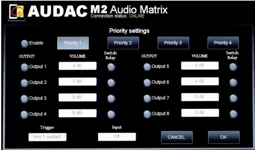
To do a priority setting first choose a channel on which the M2 will trigger your setting. Now an input should be chosen. You can select every output to which the input should be routed. For every output it is possible to set volume and toggle relay position.
