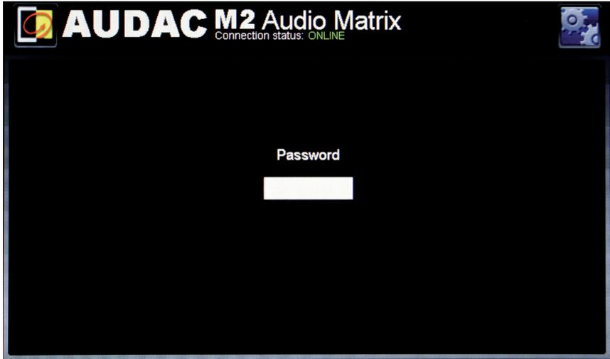
A password should be entered to get access to the M2 amplifier. There are two different access levels, administrator level and user level.
