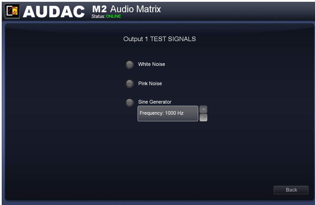
M2 Output Test Signals
